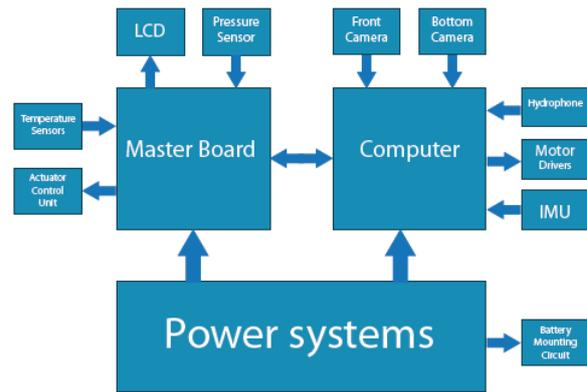
**Figure 7.** Electrical system block diagram[1]
