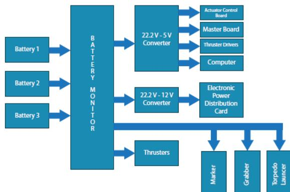
**Figure 8.** Electrical system block diagram[2]
