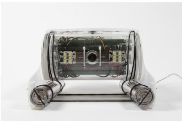
**Figure 1.** Concept design of Hybrid-AUV
