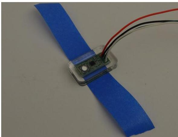
**Figure 10.** Depth sensor
