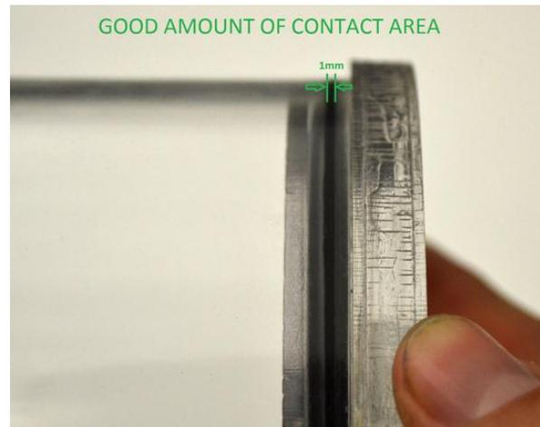
**Figure 4.** Plexi endcap with o-ring
