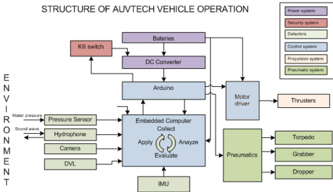
Figure 2. AUVTECH Sub-systems and their interactions.
