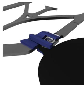
Fig 5. The 3D clip which holds end cap in place relative to the frame.
