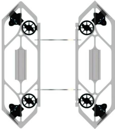
Fig 3. Prospero's final thruster layout.
