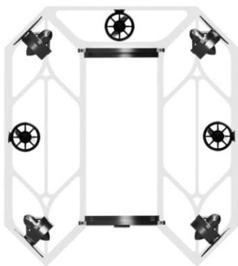
Fig 2. Prospero's initial thruster layout.
