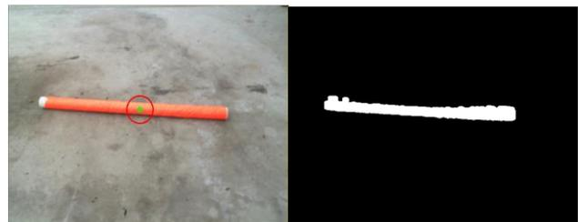
Fig 7: Color Thresholding Example. The image on the left is being processed. The image on the right is the threshold image that results when the predetermined RGB ranges includes the bright orange color.
