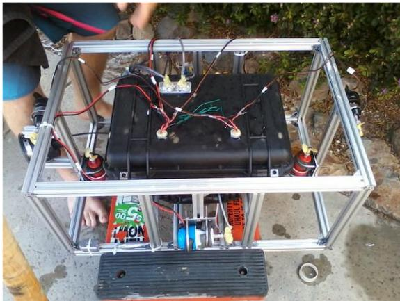
In order to reduce the number of holes in our pressure vessel, we elected to drill holes in the aluminum bolts used for heat syncing to transfer power and communication. Ensuring water tight transfer of power and communication from inside the pressure vessel to the motors and sensors was problematic; merely sealing around the jacket of the wires was not good enough, because if the jacket of the wire gets a crack in it, the water will migrate between the wire and jacket causing a leak.
