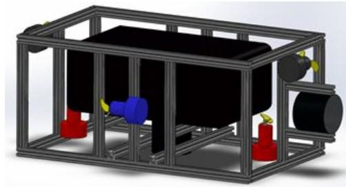
All equipment is attached to the frame via the T-slots by screws and specialized sliding bolts allowing for convenient modification through modularity. This has allowed for cost-free design changes. SolidWorks modeling was used to conduct software tests for center of mass and pressure.
