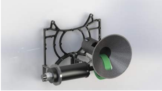
Fig. 4: CUAUV’s peg acquisition and replacement manipulator
