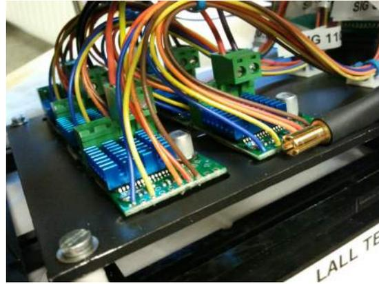
Fig. 9: Motor controller with cooling plate and heat sinks
