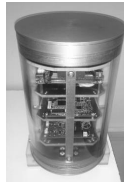
Fig 3. On board electronics inside housing.
