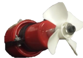
Figure 1: Customized motor; bilge pump with propeller.
