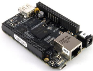
Figure 7: BeagleBone Black, central processing unit.
