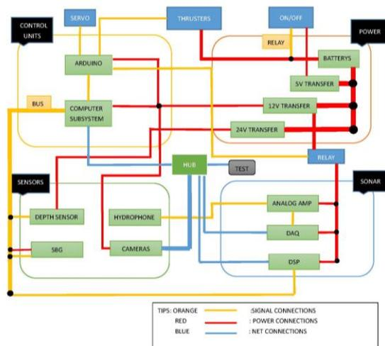
Fig 6. Block diagram of AUV's electrical systems
