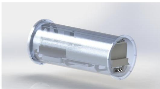
Fig 2. Main hull of NEMO II
