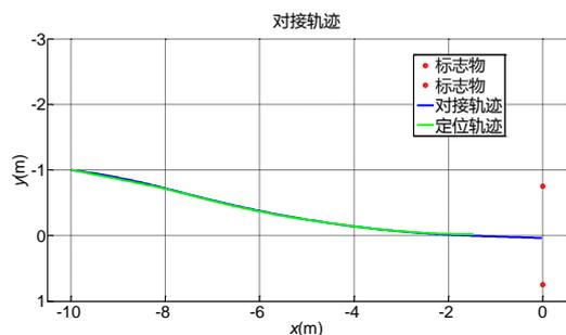
Fig 16. Certification of monocular position method, in which the green line stands for the observation and blue line stands for the trajectory of our AUV
