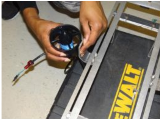
Fig. 8 Example of Thruster Modularity Along Past Platform Base
