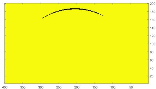
Fig 11. Two hydrophone array comparing received times to a time table generated based on expected times. The black curve represents possible locations.
