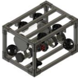
Figure 1: Box structure of the sub. Motors are not across the same plane.
