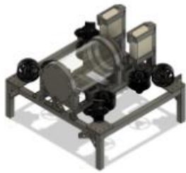
Figure 2: 80/20 bars are stacked to allow for easy addition of T-nuts into the frame with hardpoint for lifting.
