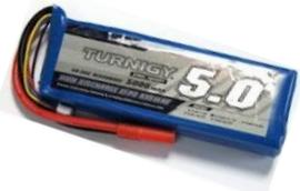
Fig 7:- 5000 mah Lipo Battery powers the Thrusters and motors
