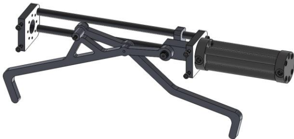
Fig 10. CAD rendering of Riptide 's claw.
