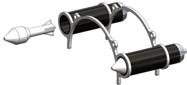
Fig 11. CAD rendering of Riptide 's torpedo launcher system, with one torpedo in resting position and one in the launched position.
