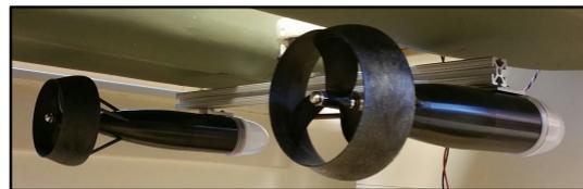
Figure 4: One of USNA RoboBoat’s moment arms holding two underwater motors.
