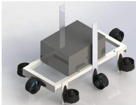
Fig 2. Redesigned Configuration with Pelican case
