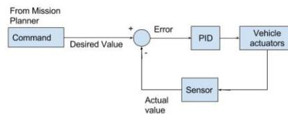
Fig 13. Simple PID controller example
