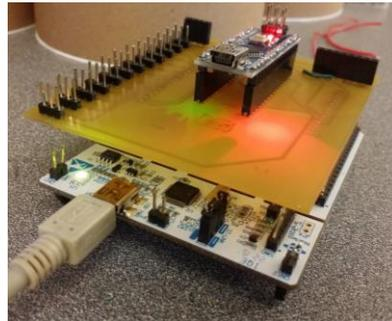
Fig 8. STM32 and control shield
