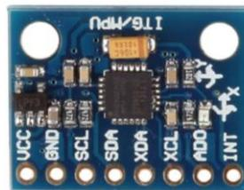
Fig 9. MPU6050 Breakout Board
