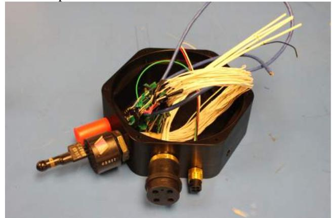
Figure 1: Bottom Endcap During Assembly
