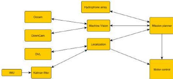
Figure 5: Software Block Diagram
