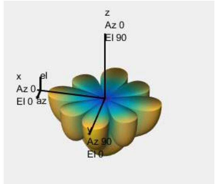
Figure 4: Hydrophone 3D Directivity Pattern at 40kHz.
