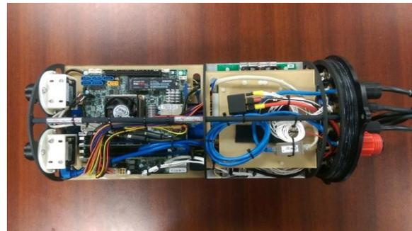
**Figure 4:** Internal electronics carriage for the main vessel. Above the tray there is easy access to PCBs and wiring, while batteries are stored below the tray
