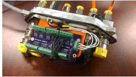
**Figure 11:** Pneumatic solenoid housing and control board
