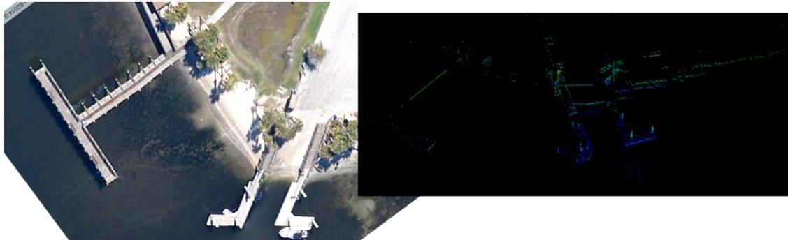
*Figure 2. Velodyne Data Showing Low IR Reflectivity from Water Areas.*
