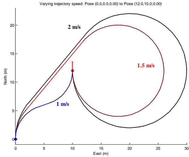
Figure 4. Trajectories at Varying Operating Speeds
