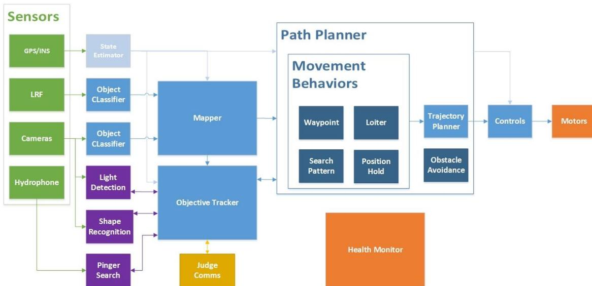
Figure 3. ERAU WAM-V Software Architecture
