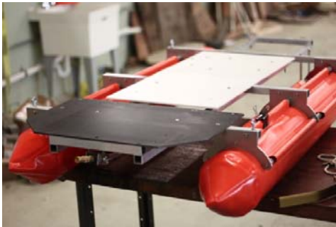
Figure 5: Assembled Hull and Frame
