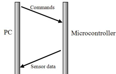
Figure 6. Data communication between PC and microcontroller
