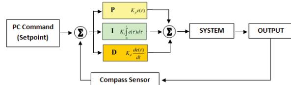
Figure 9. PID control of PENSHP
