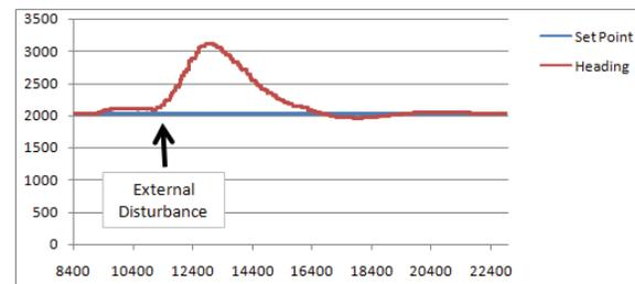
Figure 10. PID controller experiment result
