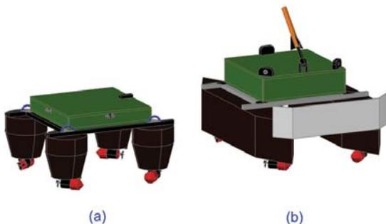
Figure 1. (a) Hull design of first generation PENSHIP, (b) New hull design of second generation PENSHIP
