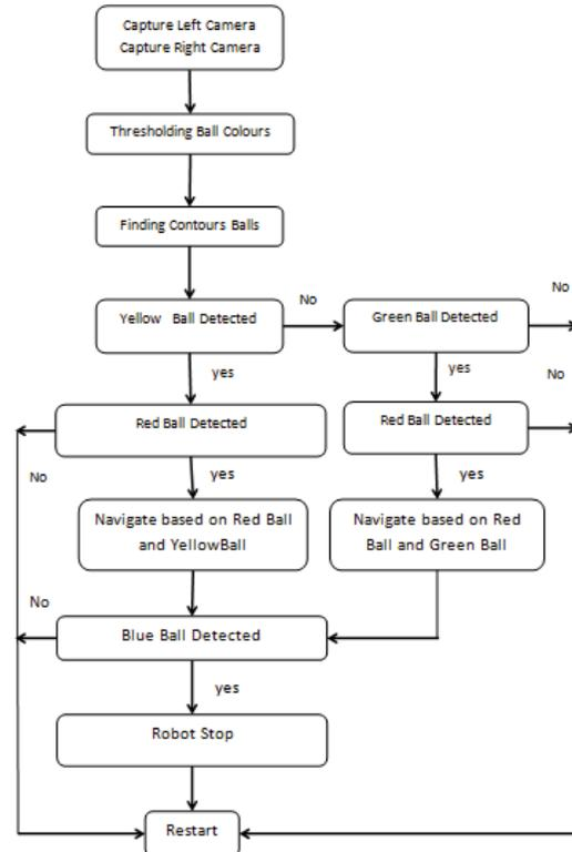
Figure 14. Ball detection algorithm of PENSHP
