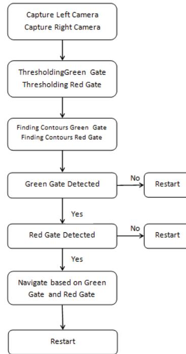
Figure 13. Gate detection algorithm of PENSHP
