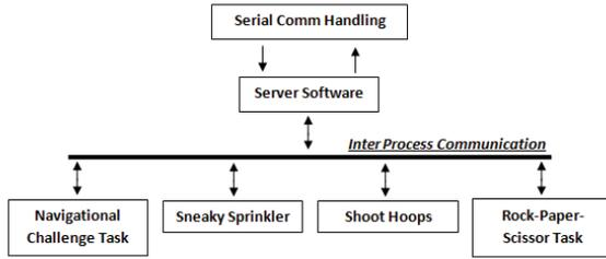
Figure 11. Process of software management for PENSHP
