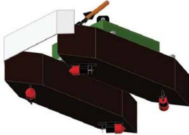
Figure 3. Motors placement of PENSHP
