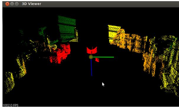
Figure 13 An example of 3D data collected from the tilting LIDAR unit. Distances have been color coded to a heat map.
