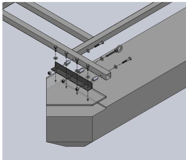
Figure 3 Pontoon with polycarbonate mounting plate configuration
