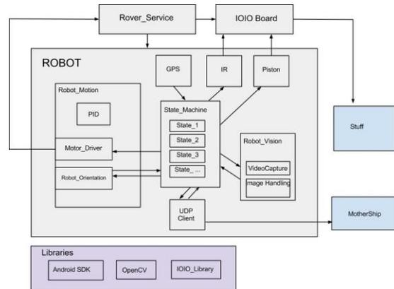
Figure 15 Rover's software diagram
