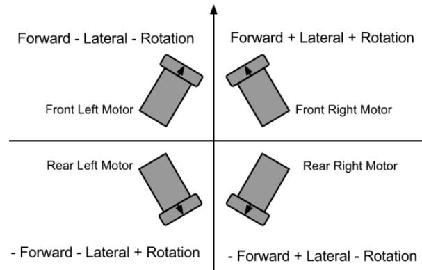
Figure 9 Illustration of motor configuration
