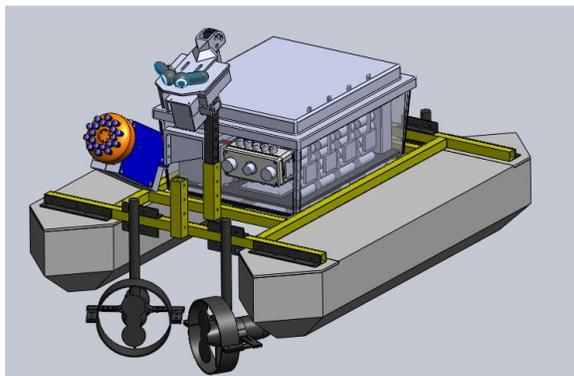
Figure 1 CAD model of Gray Goose
