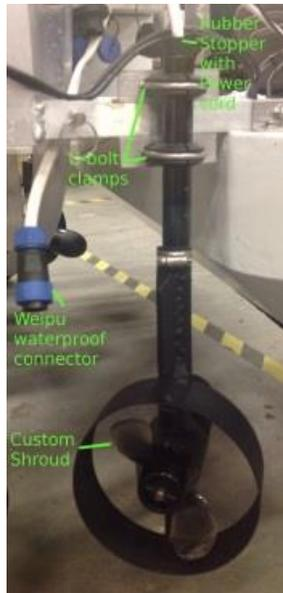
Figure 4 modified trolling motor
