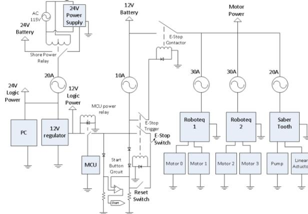
Figure 8 Power distribution diagram
