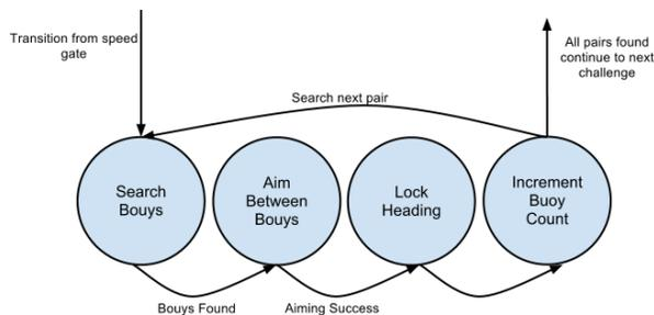
Figure 12 buoy navigation state machine example
