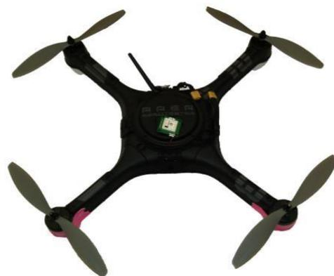
Figure 7: Aerotestra Quadrotor Frame
