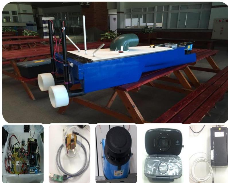
Figure 1 Diagram of overall Roboat system components
