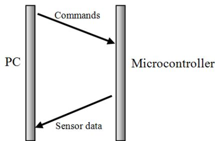
Figure 4. Data communication between PC and microcontroller
