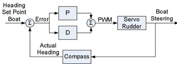
Figure 9. PD Controller design of PENSHP 2015
