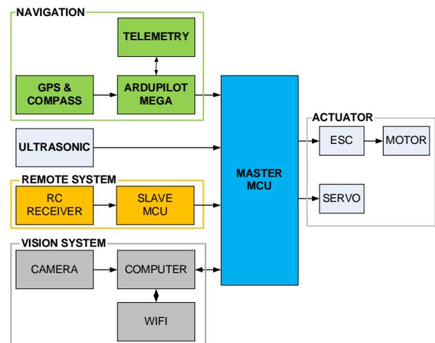
Figure 3. Hardware architecture of PENSHIP v4
