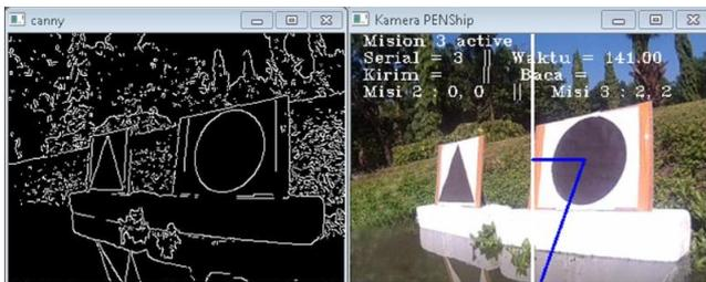
Figure 11. Symbol recognition using canny edge detector
