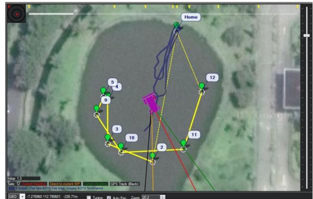
Figure 8. Visualization of PENSHP v4 waypoint navigation on mission planner monitor
