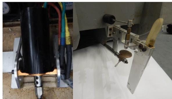
Figure 5. Actuator for steering the boat
